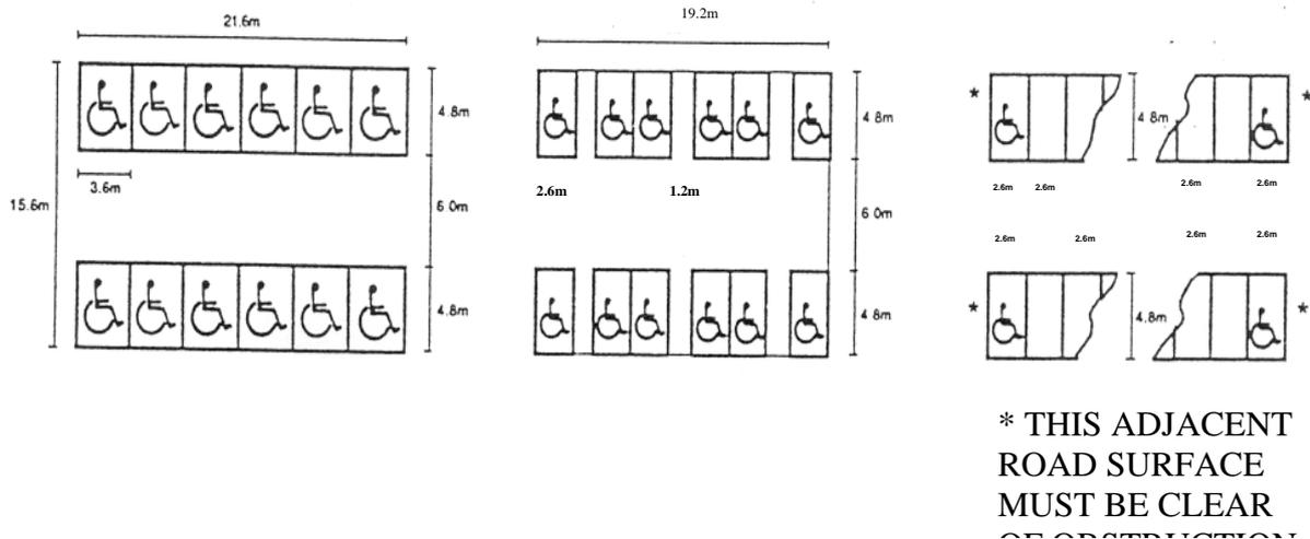
**Vehicle Bays** - The bay must be of sufficient size and be located so that the vehicle can be manoeuvred within the site, e.g. the 12m rigid lorry requires a absolute minimum of 105m<sup>2</sup> to allow it to leave a site in forward gear. Further details of good design practice can be found in appropriate Highway Authority Design Standards or 'Designing for Deliveries', Freight Transport Association 1998.
